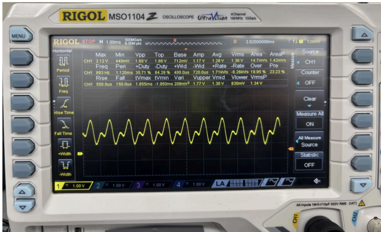
Figure 4. Output wave from microphone in noisy lab environment
