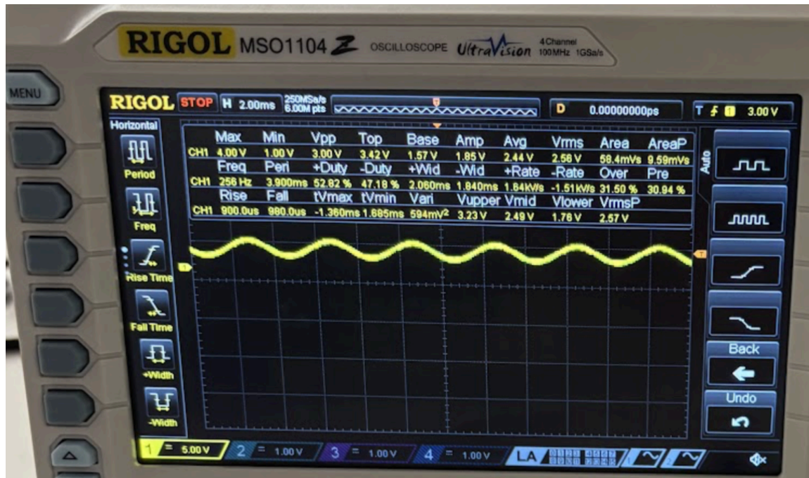
Figure 9. DAC60501 voltage output reading for desired 256Hz sine wave
